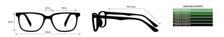
"The 17004 welding glasses have a glass green welding filter shade 2.0, 3.0, 4.0, 5.0, 6.0, 8.0, that provides torching and brazing protection. These Green torching glasses are ANSI Z87.1, EN 166 and EN 169 approved, and have CE certified lens. These welding safety glasses 17004 are made of high-quality plastic, it is a durable and lightweight wrap around frame. The 17004 welding glasses feature adjustable temple bars. These Phillips Safety torching glasses are available in black."
