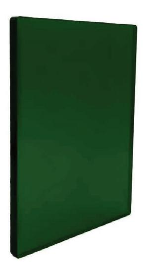
The Custom Glass Welding Window are custom glass sheets for use in welding windows or portholes for automated welding. They can be custom cut in any size sheet up to 36" x 42". These Phillips Safety glass sheets are available in shades 4, 5, 6, 8, 9, 10, 11, 12, and 14. The glass sheet thickness is 2.7mm with a tolerance of +/- 0.3mm.
