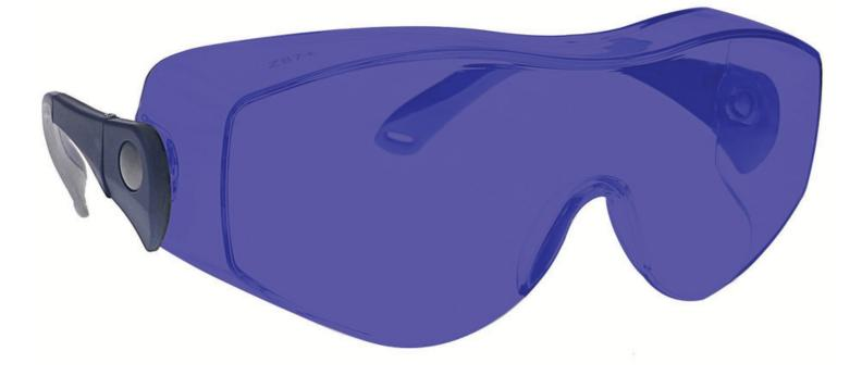
The lampworking glasses Sodium Flare Poly have a polycarbonate purple glassworking lens that provides good color recognition for soft glass. These flameworking glasses offer excellent UV blocker, good IR protection, excellent sodium flare blocker, and good clarity. Recommended for those who work with lampwork or hot glass in small pieces.
