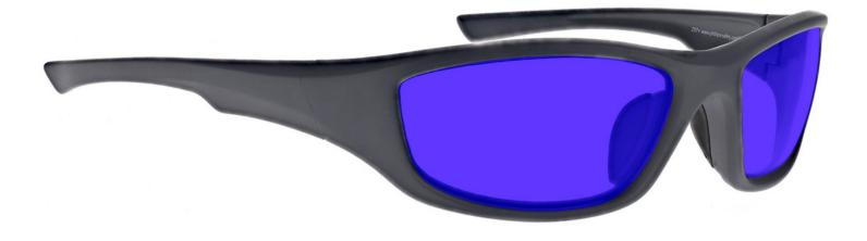
The lampworking glasses Sodium Flare Poly have a polycarbonate purple glassworking lens that provides good color recognition for soft glass. These flameworking glasses offer excellent UV blocker, good IR protection, excellent sodium flare blocker, and good clarity. Recommended for those who work with lampwork or hot glass in small pieces.
