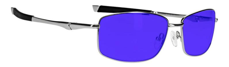
The lampworking glasses Sodium Flare Poly have a polycarbonate purple glassworking lens that provides good color recognition for soft glass. These flameworking glasses offer excellent UV blocker, good IR protection, excellent sodium flare blocker, and good clarity. Recommended for those who work with lampwork or hot glass in small pieces.
